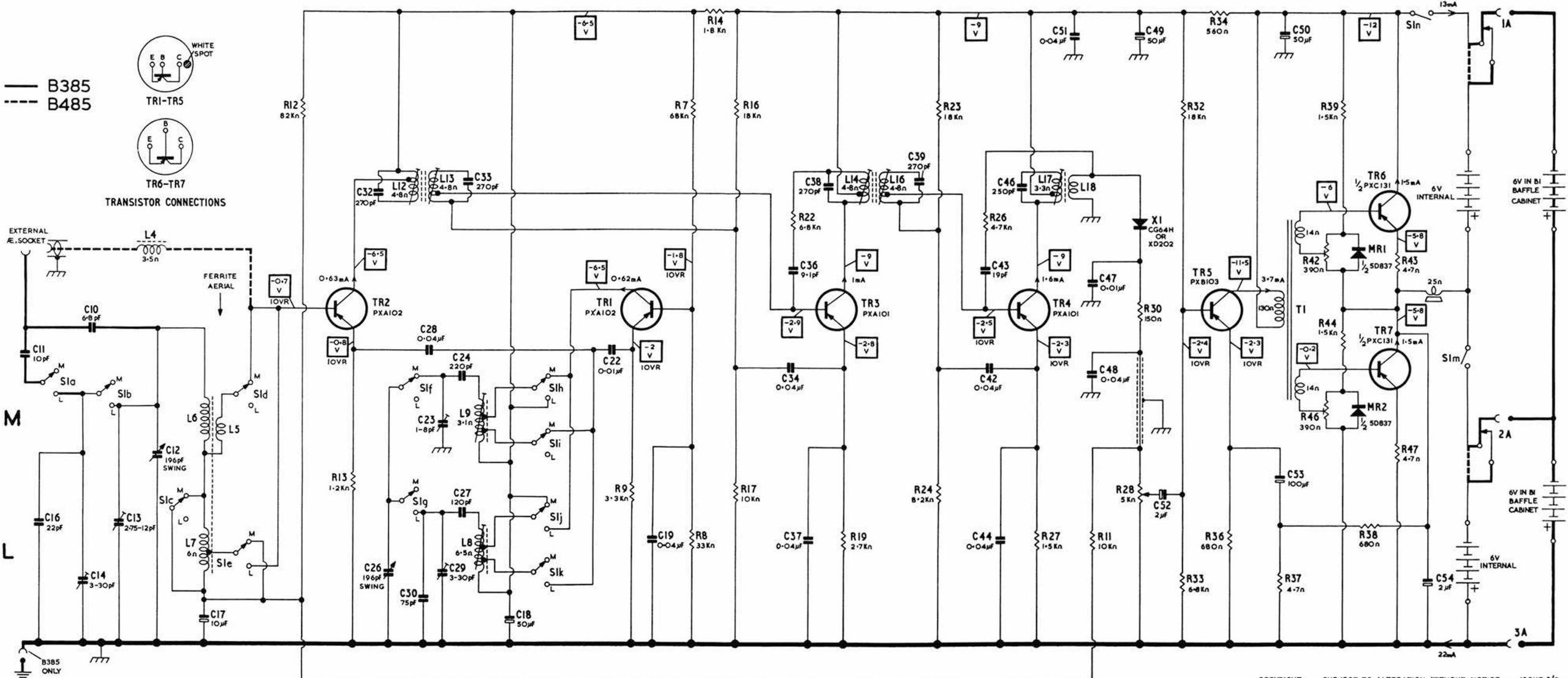
The wave-range switch is shown in the M position, and the d.c. resistance of the coils is omitted where the value is less than one ohm. Voltage and current readings were taken under no-signal conditions with the receiver switched to the M range and the
