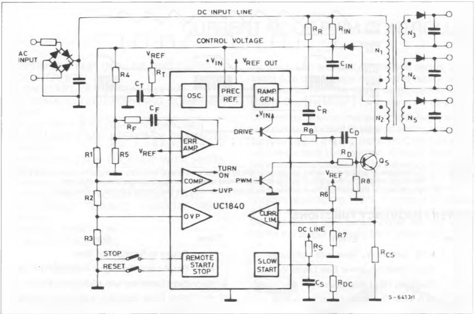
In this application [see Fig.8] complete control is maintained on the primary side. Control power is provided by  $R_{IN}$  and  $C_{IN}$  during start-up, and by a primary-referenced low voltage winding,  $N_2$ , for efficient operation after start. The error amplifier loop is closed to regulate the DC voltage from  $N_2$  with other outputs following through their magnetic coupling - a task made even easier with the UC1840's feed-forward line regulation.
