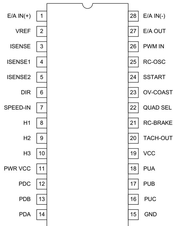
A. This pinout applies to the SOIC (DW), PLCC (Q), and LCC (L) packages (ie. pin 22 has the same function on all packages.)
