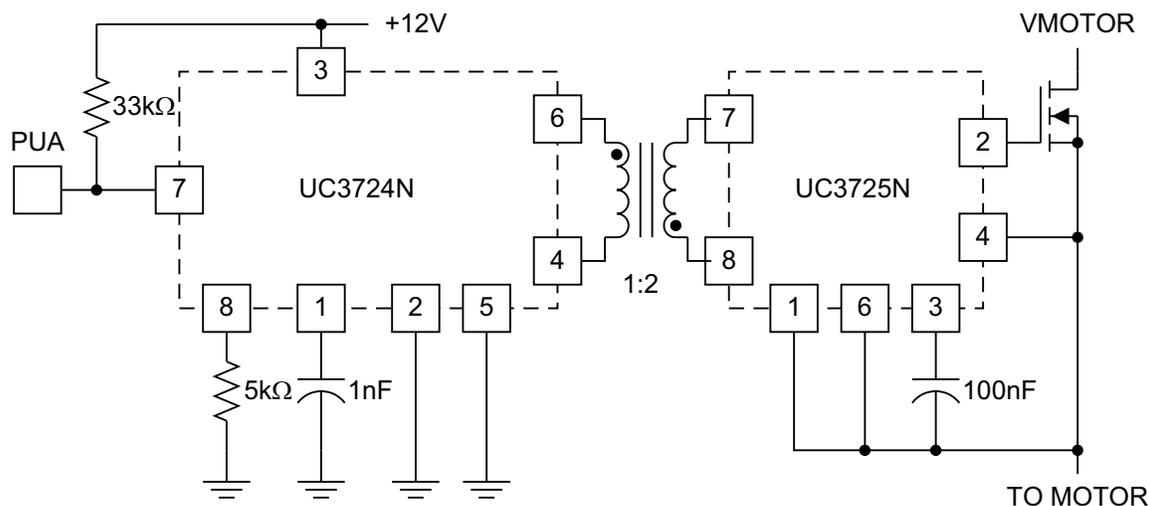
**Figure 13. Fast High-Side N-Channel Driver with Transformer Isolation**
