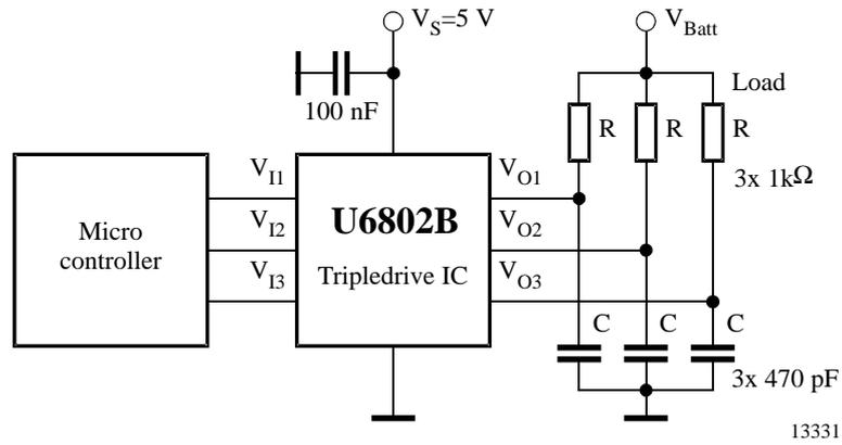
Figure 3. Application schematic
