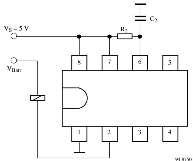
Figure 2b Basic circuit for V<sub>S</sub> = 5 V
