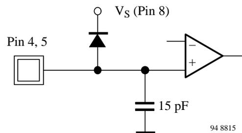
Figure 3b Input circuit Pin 4 and Pin 5
