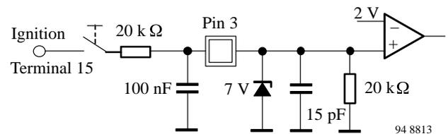
Figure 3a Input circuit for ignition (Pin 3)
