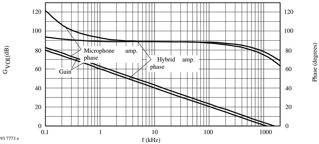
Figure 17. Microphone- and 1<sup>st</sup> hybrid amplifier open loop gain and phase versus frequency
