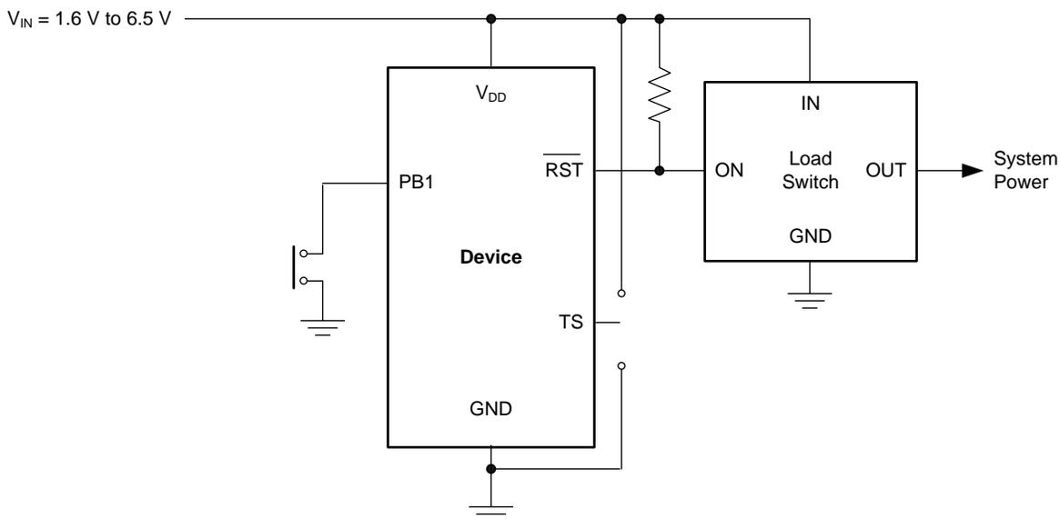
NOTE: Connect TS to  $V_{DD}$  or ground for different PB time delays.
