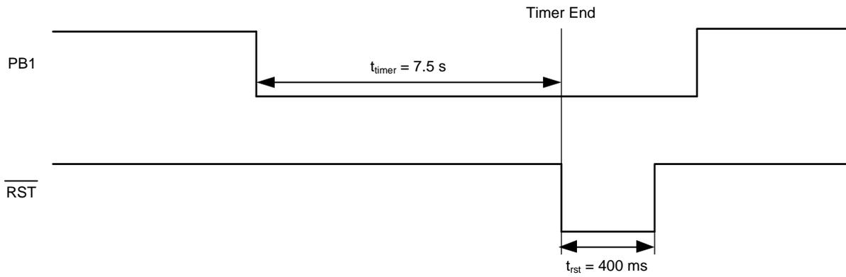
Figure 1. Timing Diagram
