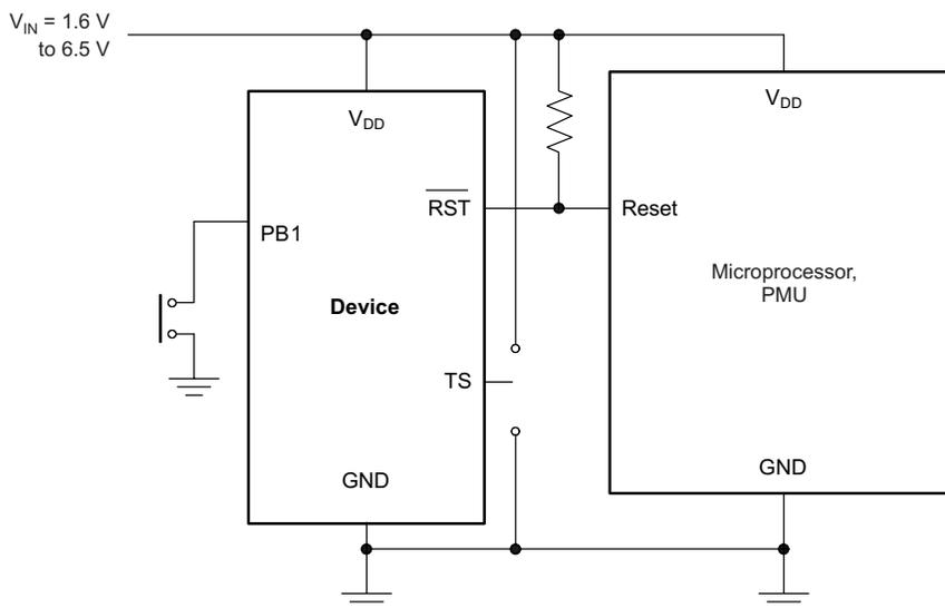
NOTE: Connect TS to  $V_{\text{DD}}$  or ground for different PB time delays.
