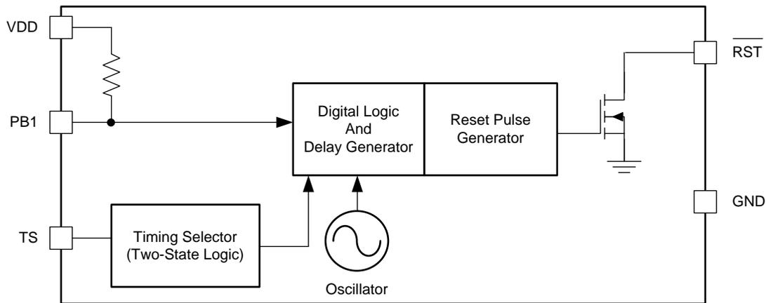
Figure 2. Block Diagram
