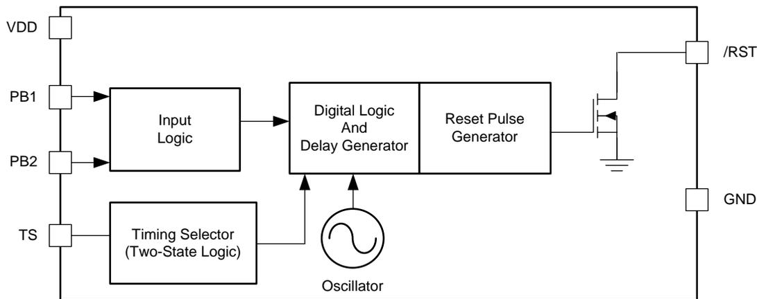
Figure 2. Block Diagram
