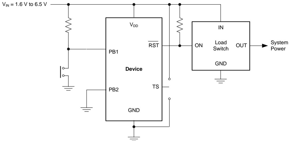
NOTE: Connect TS to  $V_{DD}$  or ground for different PB time delays. Connect one PB input to ground for use as a single channel.
