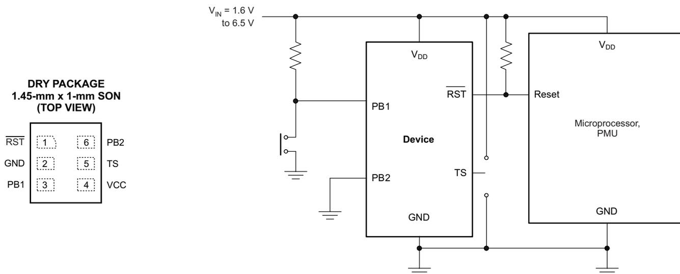
NOTE: Connect TS to  $V_{\text{DD}}$  or ground for different PB time delays. Connect one PB input to ground for use as a single channel.
