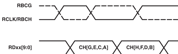
Figure 6. Multiplexed Channel Receive Timing
