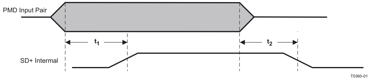
Figure 9-20. 100Base-TX Signal Detect Timing
