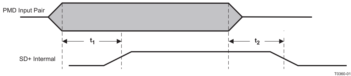
Figure 9-20. 100Base-TX Signal Detect Timing
