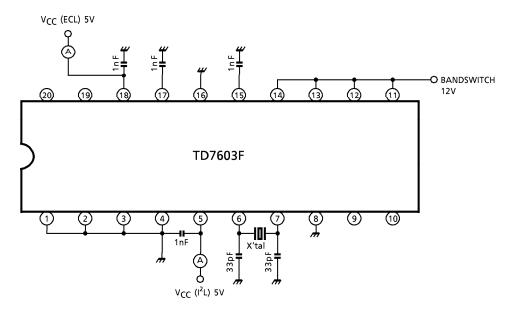
TEST CIRCUIT 3: Input sensitivity measuring circuit (Pin numbers are for the flat package.)
