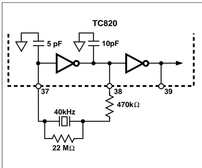
Figure 15. Suggested Crystal Oscillator Circuit
