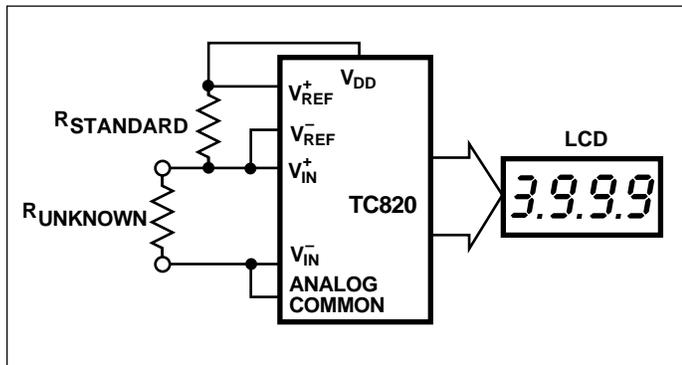
Figure 19. Low Parts Count Ratiometric Resistance Measurement
