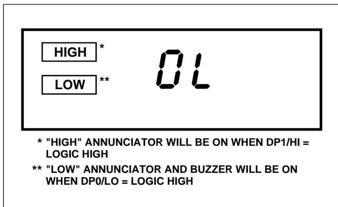
Figure 7. LCD During Logic Probe Operation
