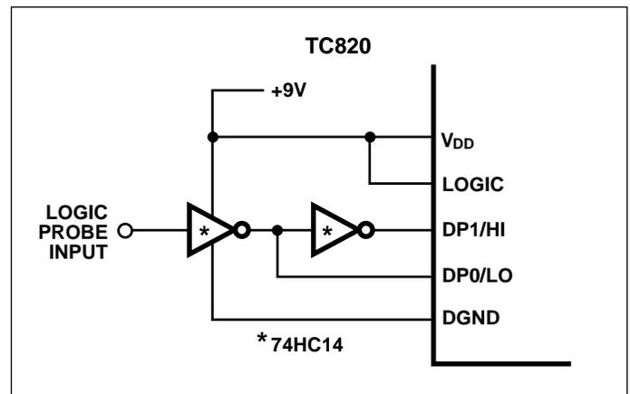
Figure 21. Simple External Logic Probe Buffer
