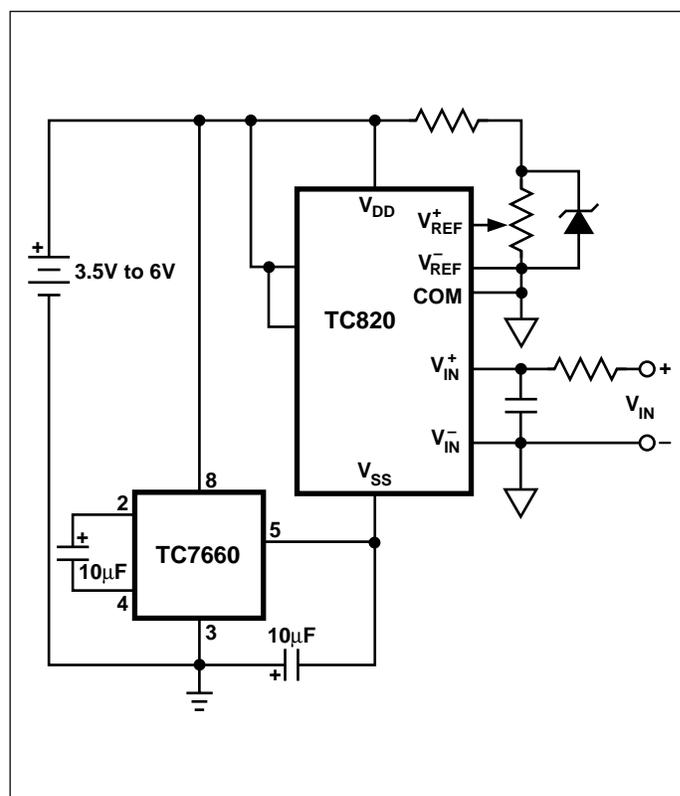
Figure 13. Powering the TC820 From a Low-Voltage Battery
