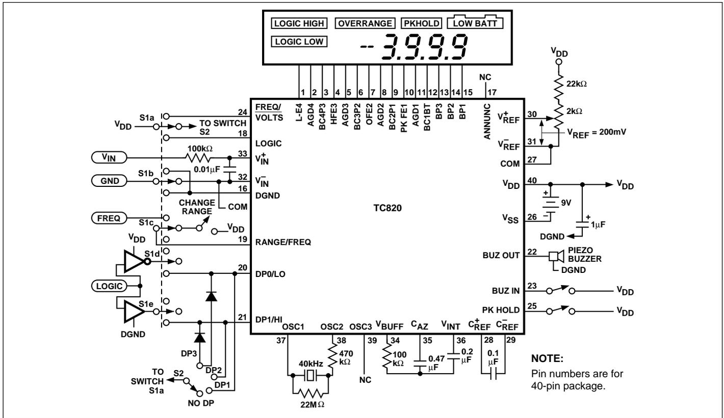
Figure 1. Typical Operating Circuit
