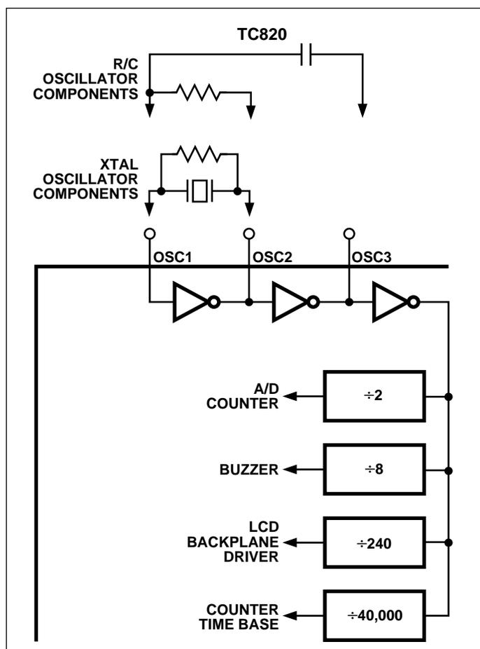
Figure 17. System Clock Generation
