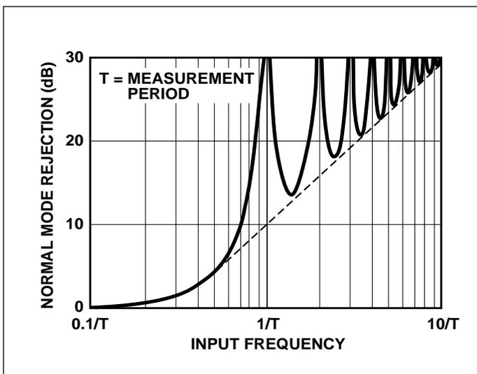
Figure 3. Normal-Mode Rejection of Dual-Slope Converter
