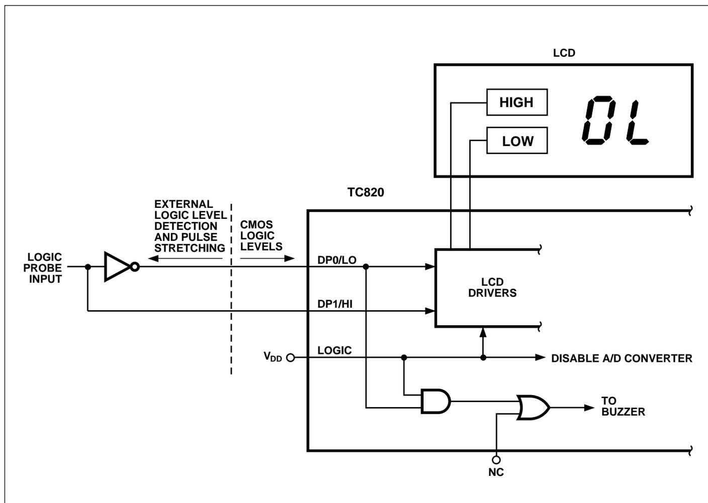
Figure 6. Logic Probe Simplified Schematic
