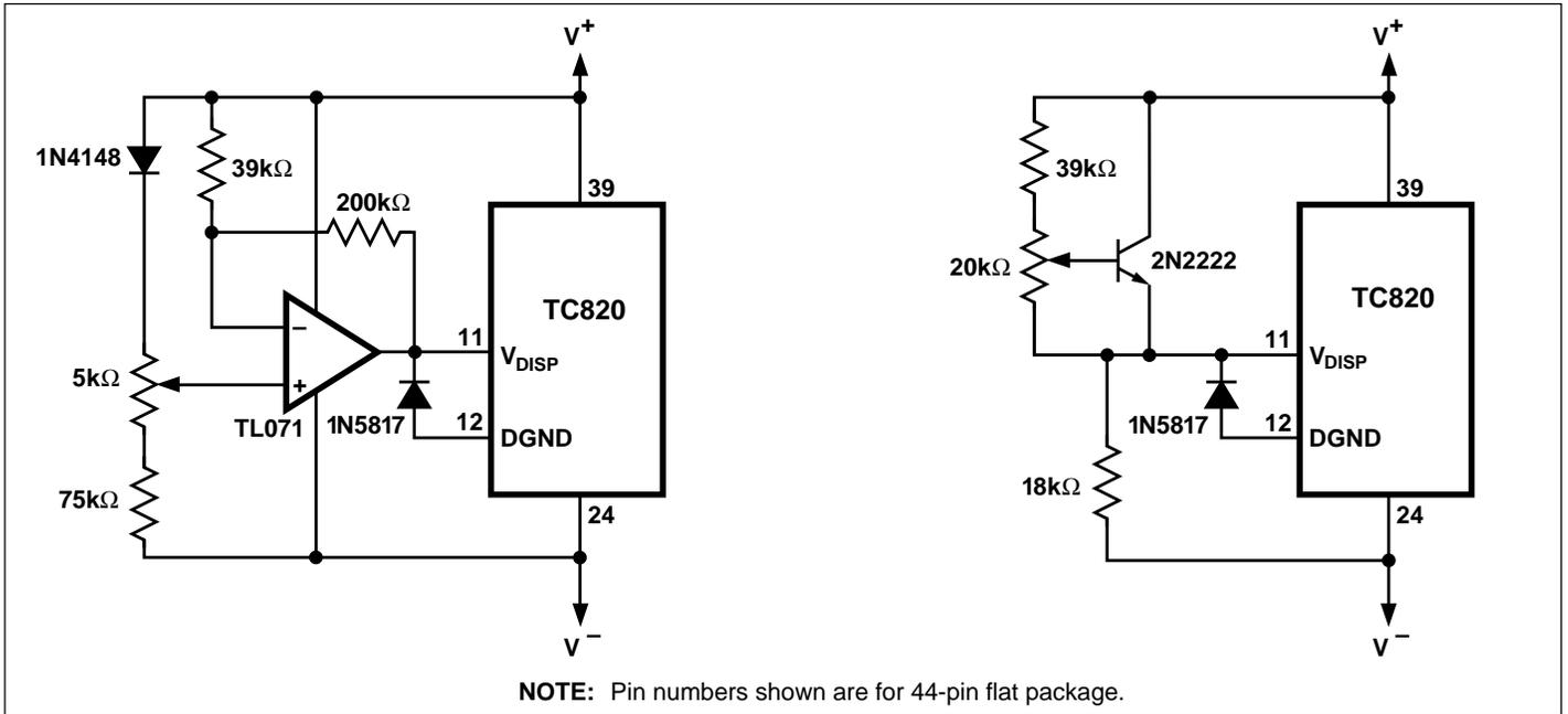
Figure 27. Temperature-Compensating Circuits
