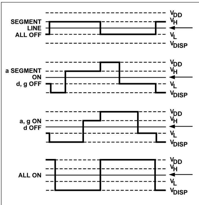
Figure 25. Typical Display Output Waveforms
