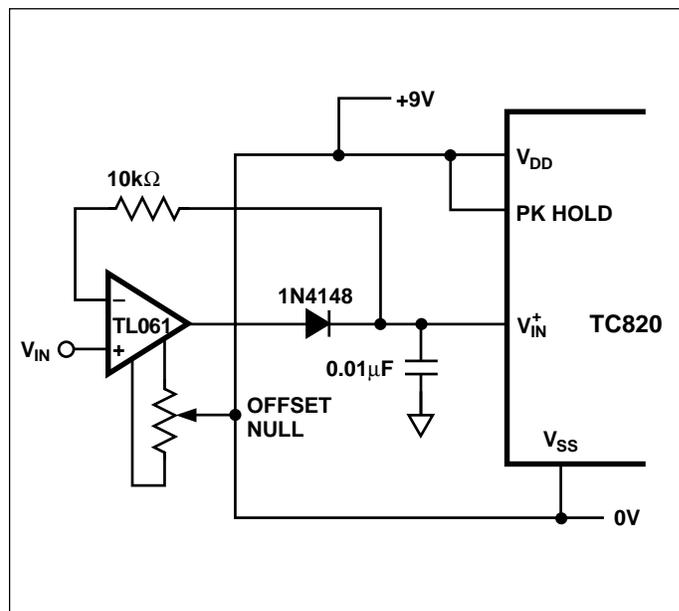
Figure 23. External Peak Detector
