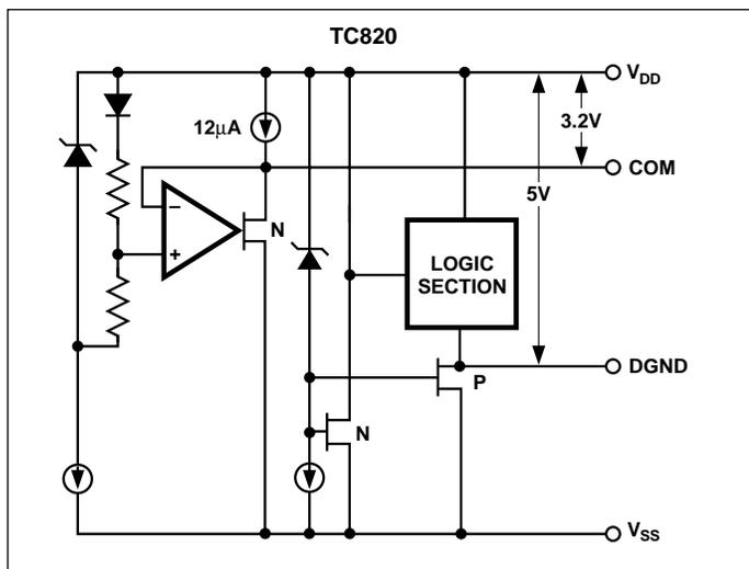
Figure 14. DGND and COM Outputs
