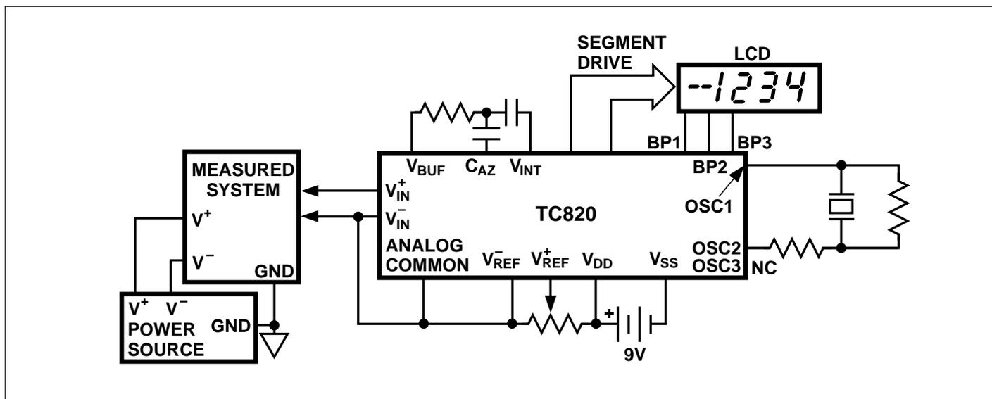
Figure 8. Common-Mode Voltage Removed in Battery Operation With  $V_{IN} = \text{Analog Common}$
