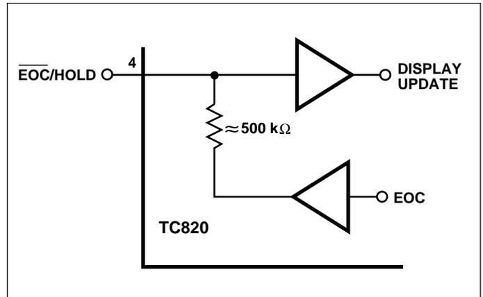
Figure 10.  $\overline{EOC}/HOLD$  Pin Schematic
