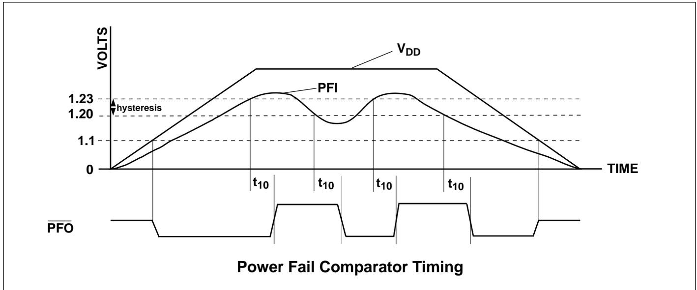
Figure 5. Power Fail Timing
