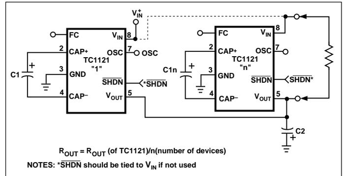
Figure 4. Paralleling TC1121s to Reduce Output Resistance
