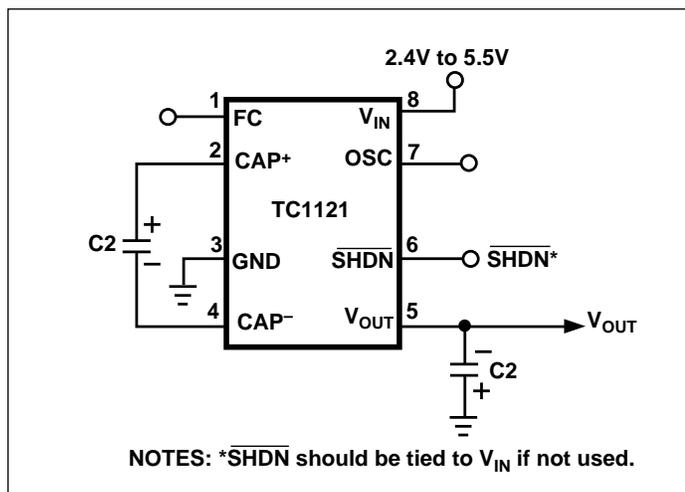
Figure 1. Charge Pump Inverter
