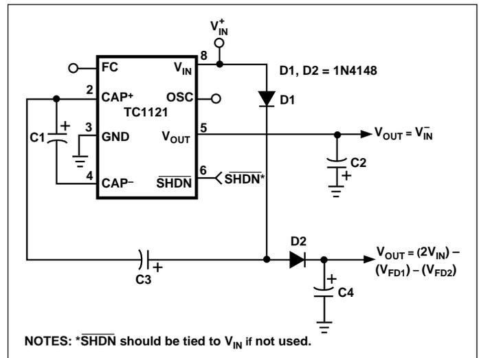
Figure 5. Combined Positive Multiplier and Negative Converter
