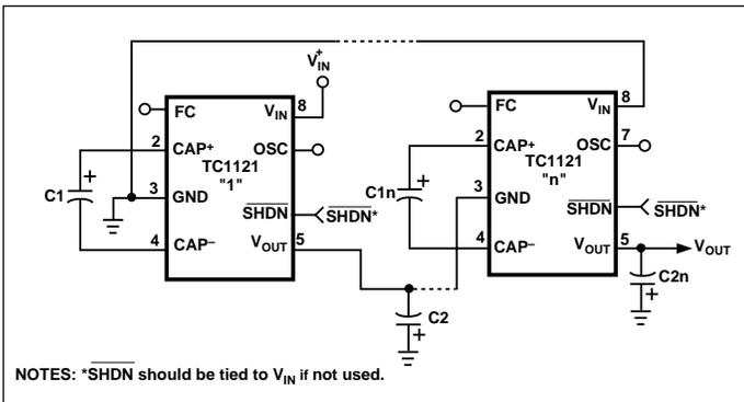
Figure 3. Cascading TC1121s to Increase Output Voltage
