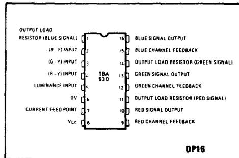
Fig. 1 Pin connections
