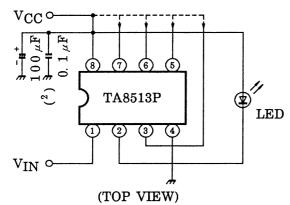
See item next figure for connection method of pins No.3, 5, 6 and 7.
