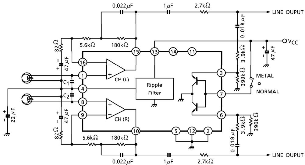
(Note) Capacitor C<sub>1</sub> and C<sub>2</sub> may be required for preventing a instability caused by the pattern layout or interference of external high frequency signal.
