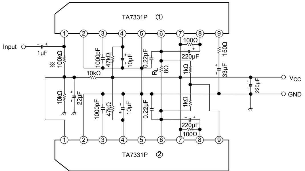
※ It is necessary to adjust to I<sub>CCQ</sub>.
