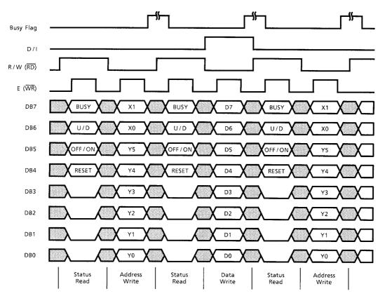
• 8-bit mode, 80-series MPU interface (80 /  $\overline{68}$  = H)
