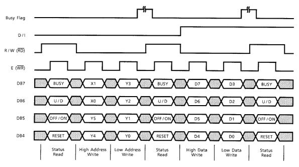
The Busy flag is set on the falling edge of the second E signal. In this mode, it is not necessary to check the Busy flag between sending the upper data nybble and sending the lower data nybble.
