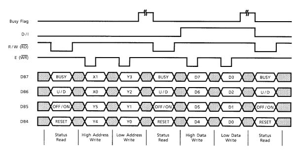
• 8-bit mode, 68-series MPU interface (80 /  $\overline{68}$  = L)
