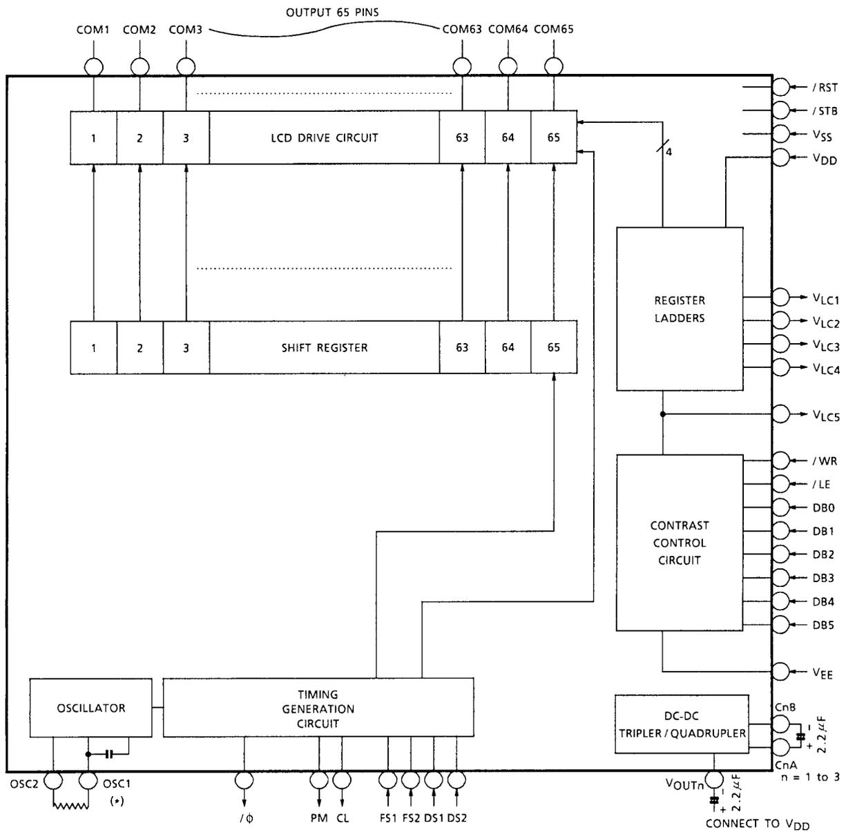
\*: When external clock operation is used, the clock should be input to OSC1.
