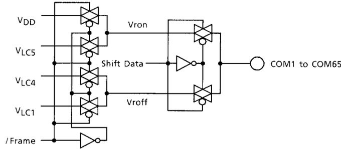
● **Resistor ladder, contrast control circuit**
