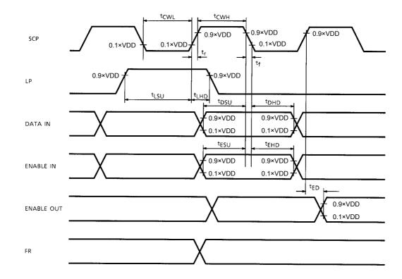
TEST CONDITIONS (Unless Otherwise Noted,  $V_{SS} = 0 V$ ,  $V_{DD} = 5 V \pm 10\%$ ,  $V_{LC5} = 0 V$ , Ta = -20 to 75°C)
