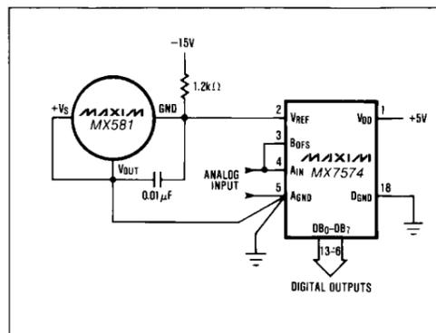
Figure 8. Negative 10V Reference for CMOS A/D Converter
