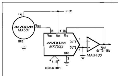
Figure 7. Low Power 10 Bit CMOS DAC Connection
