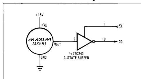
Figure 9. MX581 Microprocessor Interface
