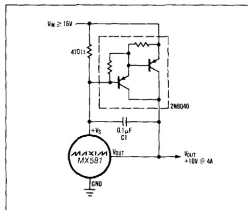
Figure 3. High Current Precision Supply
