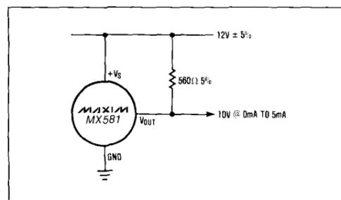
Figure 4. 12-Volt Supply Connection
