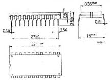
Dual in-line ceramic frit seal package (M760A)
