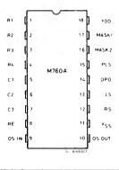
Dual in-line ceramic frit seal package (M760)
