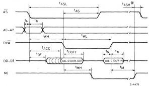
\* The first falling edge of AS following the end of a modify cycle must occur at least t<sub>ASH</sub> after the positive edge of ME.
