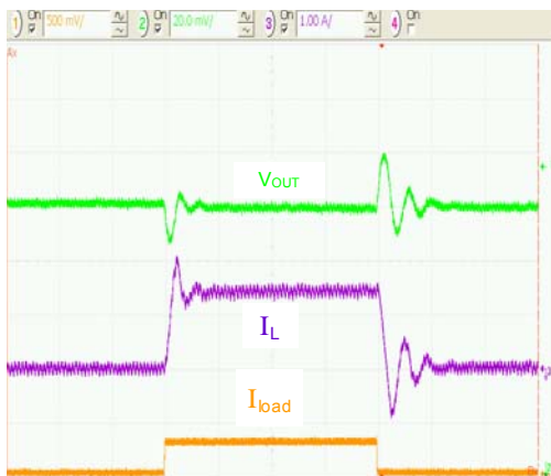
Figure 15. MODE=1, 100 mA to 1.5 A to 100 mA, 5 \mu\text{s}/\text{div} .
