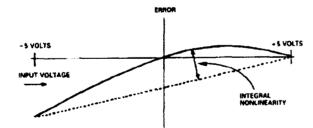
Figure 2. Relative Accuracy and Integral Nonlinearity when Calibrated
