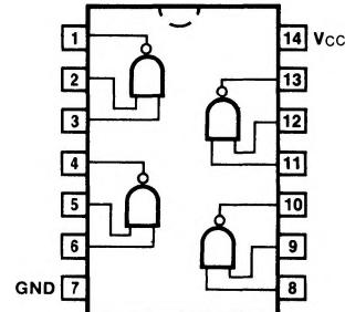
**INPUT LOADING/FAN-OUT:** See Section 3 for U.L. definitions
